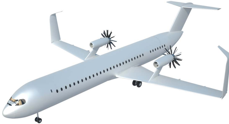
Fig. 83 Albatross in docking mode with wings folded
